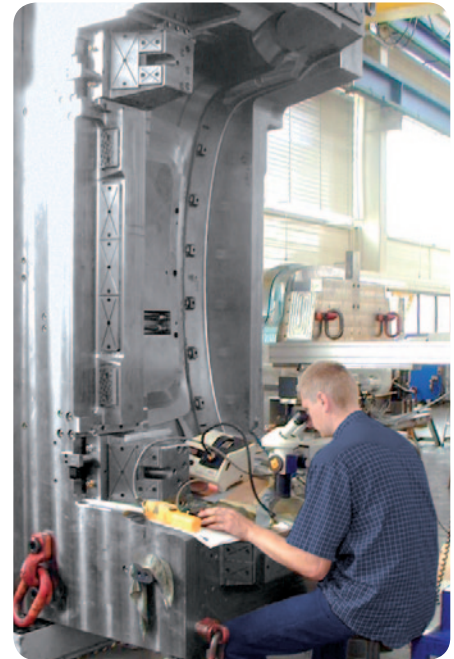
Processing of a 20 t mold for the production of automobile bumpers
